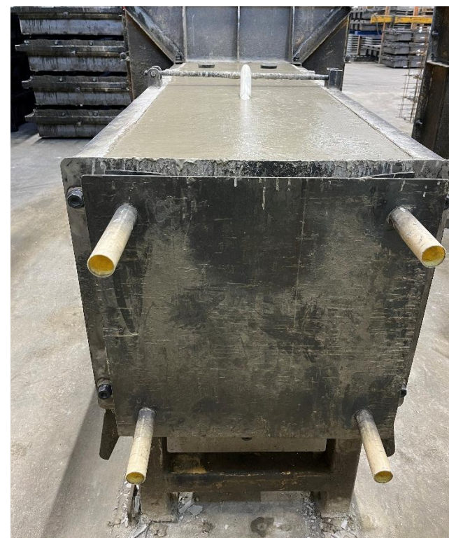
Concrete foundation for overhead contact wires (Kontaktledningsfundament i betong) – S:t Eriks AB
