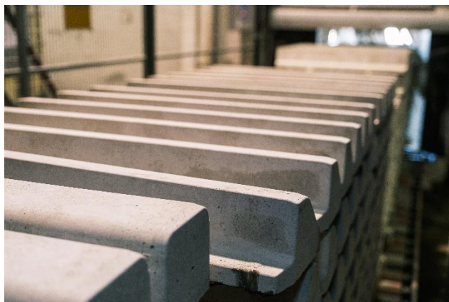
Kerbstones for streets recently produced in the factory.
