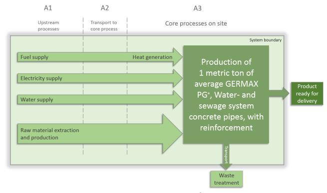
Figure 2. Flow diagram of the assessed life cycle stages for GERMAX PG®, beginning with raw material extraction and production, followed by transport from supplier to site and finally manufacturing at the core sites.
